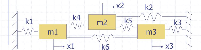
m1=0.5 Kg m2=1.0 Kg m3=1.5 Kg k1=k2=k3=k4=k5=k6=1000 N/m
